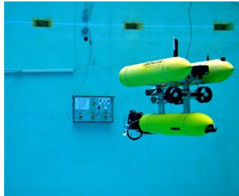
Girona 500 I-AUV (ECA CSIP Manipulator)
